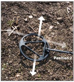
Sweep the detector from Position 1 over the anomaly, then go to Position 2 and repeat the process. If necessary, repeat swinging from a third position. When this is done from different sides, you will know exactly how long and wide the detected object is.
