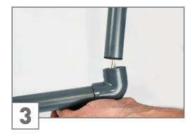
Assemble the coil by putting each end into the adjacent corner piece.
