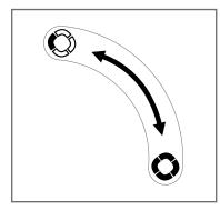
**Sensitivity Knob** (gray cap): This knob is used to regulate the sensitivity of the Search Coil. The higher the sensitivity the deeper you may find underground objects but the more noise and disturbances you may receive alongside metal signals.
