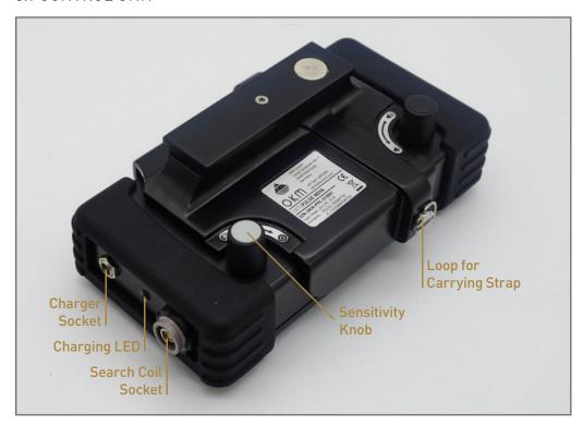
**Charger Socket / Charging LED:** When the internal battery is too low – which is signaled by a low triple tone at increasingly shorter intervals – you have to recharge it by connecting the appropriate Power Charger to the Charger Socket. As long as charging is in progress, the Charging LED is **orange**. As soon as the Charging LED turns off, the battery is fully charged. Complete details about charging the unit you will find in chapter "4.1 Charging the Control Unit" on page 13.
