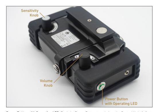
**Power Button with Operating LED:** Push the Power Button to switch on the Control Unit. At first, the Operating LED starts blinking for about 2 seconds before it remains **green** permanently. If the LED blinks rapidly before turning off, the internal battery is too low and must be charged (see chapter "4.1 Charging the Control Unit" on page 13).
