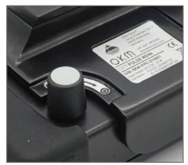
Push and hold the Sensitivity Knob of the Control Unit to start a new ground balance.
