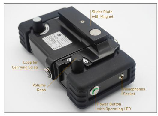
**Slider Plate:** This part is used to mount the Control Unit to the Telescopic Rod. Thanks to the embedded magnet, the Control Unit will keep in place when attached. Read chapter "4.2 Mounting the Control Unit" on page 14 to learn more about assembling and disassembling the Control Unit to the Telescopic Rod.
