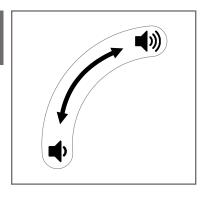
**Volume Knob** (black cap): This knob regulates the volume of the acoustic output. Turning the knob to the left lowers the volume, turning it to the right raises the volume. If the value reaches its minimum or maximum, additional turning in the same direction will have no decreasing or increasing effect. In this case, you will hear a double tone that indicates you reached the end of the adjustment range.
