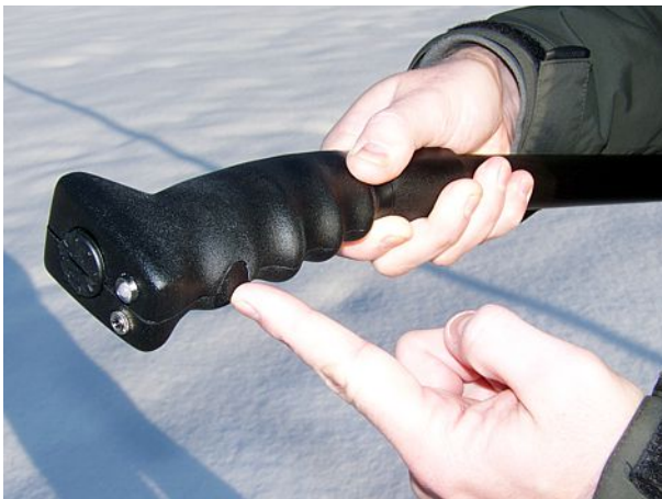
Figure 5.3: Turning on the telescopic antenna
