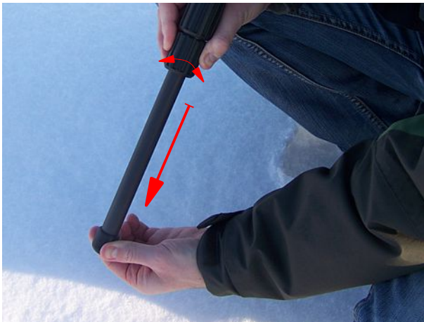
Figure 5.2: Extend the telescopic antenna
