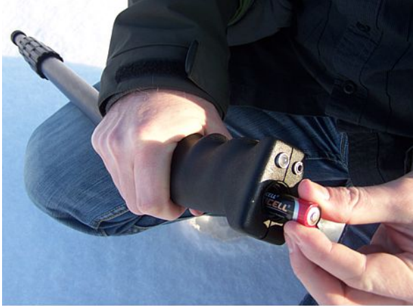
Figure 5.1: Insert the batteries into the telescopic antenna
