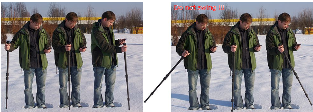
Figure 7.13: Pin-pointing with the telescopic antenna
