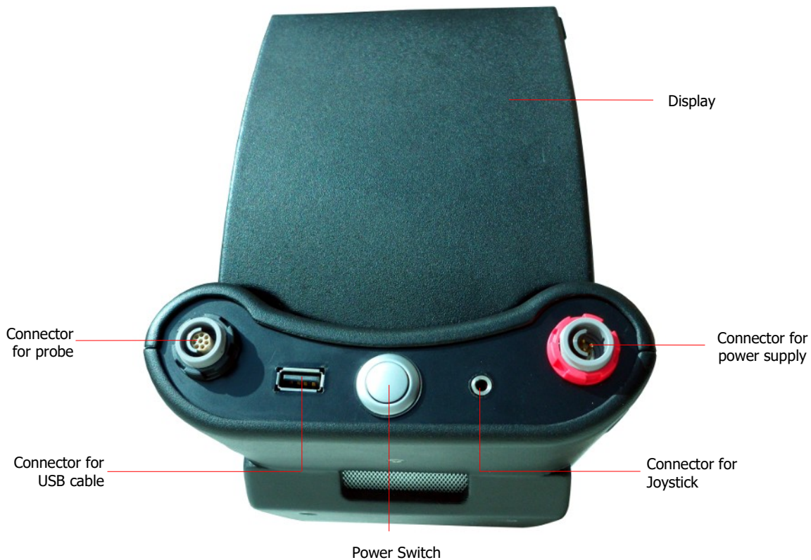
Illustration 6.3: Control unit, rear view
